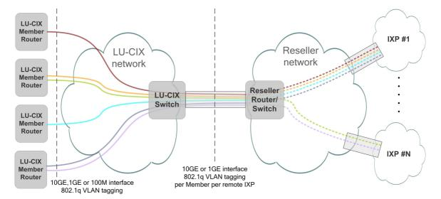
Member and LU-CIX network interconnection is based on 802.3 Ethernet protocol with 802.1q VLAN tagging. Special care has to be taken when specifying the applicable VLAN IDs to guaranty compatibility with remote IX services if VLAN translation is not provided by Member.
